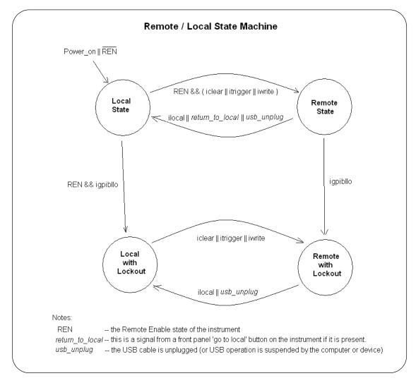
The following SICL functions are used to control the Remote/Local state transitions in USBTMC-USB488 devices sessions. (See the *SICL Online Help* for specific information on these functions.)
